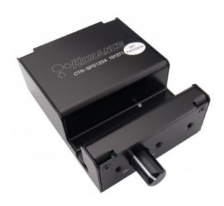
The Koolance CTR-SPD1224M uses voltage control to throttle speeds for 12V DC pumps or fans. With a jumper setting, it will also step-up and throttle voltage for 24V DC devices. A 12V DC input is required.
