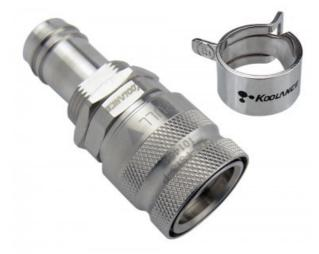
Koolance patented quick disconnect no-spill coupling with automatic shutoff. 13mm (1/2in) ID female panel-mountable hose barb with clamp for 16mm OD (5/8in). It will only fit a Koolance QD3 male quick disconnect.
