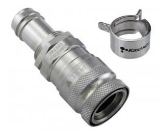
Koolance patented quick disconnect no-spill coupling with automatic shutoff. 13mm (1/2in) ID female panel-mountable hose barb with clamp for 16mm OD (5/8in). It will only fit a Koolance QD3H male quick disconnect.
