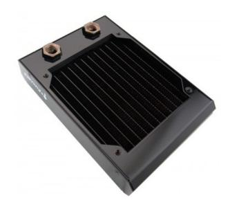
HX-CU420VS is a low profile copper core radiator designed for one 120mm fan. With a fin density of 20 FPI (fins per inch), it is optimized for quieter air flow ranges. It has a dual pass coolant design, and is G 1/4 BSPP (parallel) thread for hose fittings. 30mm (1.18") long mounting screws are included for 25mm thick fans (see Koolance <u>radiator screw packs</u> for additional options).
