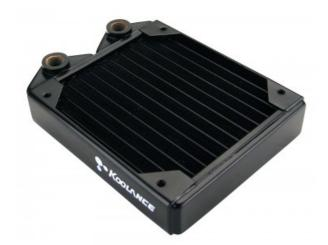
HX-CU420V is a low profile copper core radiator designed for one 120mm fan. With a fin density of 30 FPI (fins per inch), it offers best performance with higher air flow. It has a dual pass coolant design, and is G 1/4 BSPP (parallel) thread for hose fittings. 30mm (1.18") long mounting screws are included for 25mm thick fans (see Koolance <u>radiator screw packs</u> for additional options).
