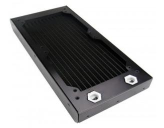
HX-720 is a low profile aluminum radiator designed for two 120mm fans. With a fin density of 18 FPI (fins per inch), it is optimized for quieter air flow ranges. It has a dual pass coolant design, and is G 1/4 BSPP (parallel) thread for hose fittings. 30mm (1.18") long mounting screws are included for 25mm thick fans (see Koolance <u>radiator screw packs</u> for additional options).
