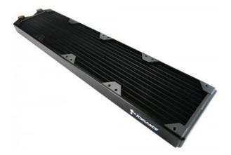
HX-CU1320V is a low profile copper core radiator designed for four 120mm fans. With a fin density of 30 FPI (fins per inch), it offers best performance with higher air flow. It has a dual pass coolant design, and is G 1/4 BSPP (parallel) thread for hose fittings. 30mm (1.18") long mounting screws are included for 25mm thick fans (see Koolance <u>radiator</u> <u>screw packs</u> for additional options).
