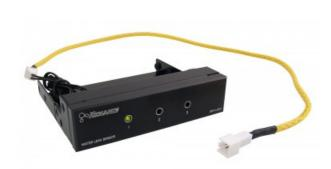
The Koolance SEN-LK001 offers leak detection for very small amounts of water. Housed in a 3.5in drive bay profile, the electronic circuit can monitor up to three separate leak sensing cables. One 46cm (18in) long sensing cable is included, which can be increased. Powered by 12VDC from a computer power supply connection.
