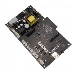
The Koolance TMS-205 thermal management system provides convenient software control over features found in many Koolance systems: temperature feedback, pump speeds, and fan speeds. In addition to these basic functions, however, are a wealth of extra capabilities!
