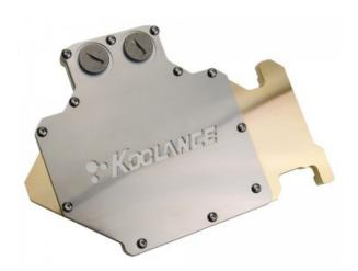
The Koolance VID-279 is a combined GPU and memory cooler for high-end video cooling of GeForce 8800GT 512MB (65nm) and 8800GTS 512MB (65nm) in single or multi video configurations. It combines a full gold-plated solid copper cooler which targets all primary heat-producing regions of the 8800, including the voltage regulators.
