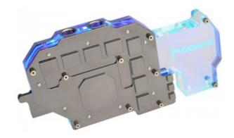
The new Koolance VID-398GX2 is a combined GPU and memory cooler for high-end water cooling of NVIDIA GeForce 9800 GX2 cards in single or multi video configurations. It combines double-sided, solid copper cold plates, nickel plating, and a thick acrylic jacket. This product is "sandwiched" between the 9800 GX2's dual video circuit boards.
