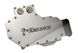
The Koolance VID-485 is a combined GPU and memory block for high-end water cooling of ATI Radeon HD 4850 video cards in single or multi video configurations. It combines a full nickel-plated solid copper cooler which targets all primary heat-producing regions of the HD 4850 (including the voltage regulators). An acrylic lid allows coolant visibility under the logo.
