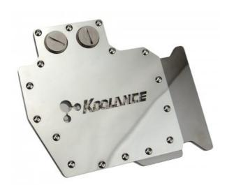
The Koolance VID-487 is a combined GPU and memory block for high-end water cooling of ATI Radeon HD 4870 and HD 4890 video cards in single or multi video configurations. It combines a full nickel-plated solid copper cooler which targets all primary heat-producing regions of the HD 4870 and 4890 (including the voltage regulators). An acrylic lid allows coolant visibility under the logo.
