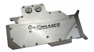
The Koolance VID-487X2 is a combined GPU and memory block for high-end water cooling of ATI Radeon HD 4870 X2 video cards in single or multi video configurations. It combines a full nickel-plated solid copper cooler which targets all primary heat-producing regions of the HD 4870 X2 (including the voltage regulators). An acrylic lid allows coolant visibility under the logo.
