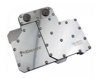
The Koolance VID-AR587T2 is a combined GPU and memory block for high-end water cooling of **revised layout** ATI Radeon HD 5870 video cards (such as the Sapphire Vapor-X 100281VX-2SR) in single or multi video configurations. It utilizes a high-performance microfin design (0.5mm) made of solid copper with anti-corrosive nickel plating. The cooler targets all primary heat-producing regions of the HD 5870, including the voltage regulators.
