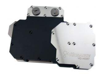
The Koolance VID-AR697 is a full coverage video block for water cooling AMD Radeon HD 6970 and HD 6950 cards in single and multi video card configurations. It utilizes a high-performance microfin (0.5mm) design made of solid copper with anti-corrosive nickel plating.
