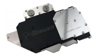
The Koolance VID-AR797 is a full coverage video block for water cooling AMD Radeon HD 7970 cards in single and multi video card configurations. It utilizes a high-performance microfin (0.5mm) design made of solid copper with anti-corrosive nickel plating.
