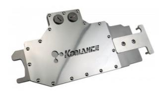
The new Koolance VID-NX275 is a combined GPU and memory cooler for high-end video cooling of NVIDIA GeForce GTX 275 cards in single or multi video configurations. It combines a full nickel-plated solid copper cooler which targets all primary heat-producing regions of the GTX 275 (including the voltage regulators). An acrylic lid allows coolant visibility under the logo.
