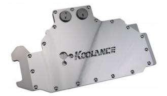
The new Koolance VID-NX285 is a combined GPU and memory cooler for high-end video cooling of NVIDIA GeForce GTX 285 1GB cards in single or multi video configurations. It combines a full nickel-plated solid copper cooler which targets all primary heat-producing regions of the GTX 285 (including the voltage regulators). An acrylic lid allows coolant visibility under the logo.
