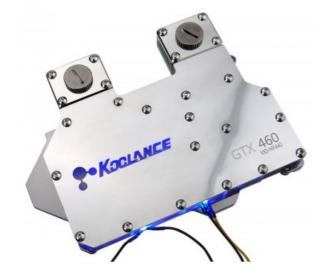
The Koolance VID-NX460 is a full coverage video block for water cooling NVIDIA GeForce GTX 460 cards in single and multi video card configurations. It utilizes a high-performance microfin (0.5mm) design made of solid copper with anti-corrosive nickel plating. The top stainless steel cover plate protects an LED illuminated acrylic lid.
