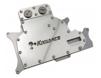
The Koolance VID-NX470 is a combined GPU and memory block for water cooling NVIDIA GTX 470 and GTX 465 video cards in single and multi video configurations. It utilizes a high-performance microfin (0.5mm) design made of solid copper with anti-corrosive nickel plating. The cooler targets all primary heat-producing regions of the GTX 470, including the voltage regulators. The top stainless steel cover plate protects an acrylic lid.
