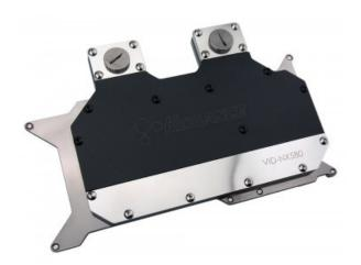
The Koolance VID-NX580 is a full coverage video block for water cooling NVIDIA GeForce GTX 580 and GTX 570 cards in single and multi video card configurations. It utilizes a high-performance microfin (0.5mm) design made of solid copper with anti-corrosive nickel plating.
