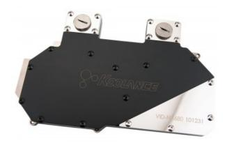
The Koolance VID-NX680 is a full coverage video block for water cooling NVIDIA GeForce GTX 680 cards in single and multi video card configurations. It utilizes a high-performance microfin (0.5mm) design made of solid copper with anticorrosive nickel plating.
