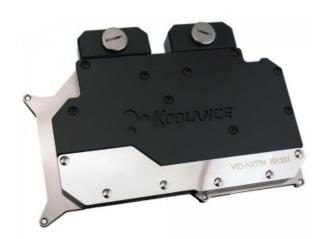
The Koolance VID-NXTTN is a full coverage video block for water cooling NVIDIA GeForce GTX TITAN and NVIDIA reference GTX 780 cards in single and multi video card configurations. It utilizes a high-performance microfin (0.5mm) design made of solid copper with anti-corrosive nickel plating. An aluminum back plate is included to handle the rear memory chips.
