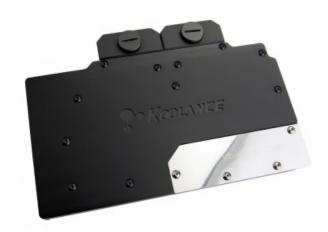
The Koolance VID-NX1080 is a full coverage video block for water cooling NVIDIA reference GeForce GTX 1080 and GTX 1070 cards in single and multi video card configurations. It utilizes a high-performance microfin (0.5mm) design made of solid copper with anti-corrosive nickel plating. This version has an acetal top. Thermal interface material and mounting hardware are included. Tube fitting threads are G 1/4 BSPP.
