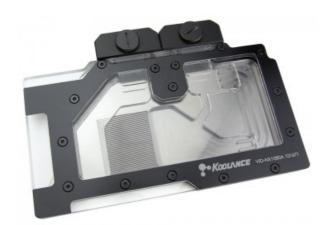
The Koolance VID-NX1080 is a full coverage video block for water cooling NVIDIA reference GeForce GTX 1080 and GTX 1070 cards in single and multi video card configurations. It utilizes a high-performance microfin (0.5mm) design made of solid copper with anti-corrosive nickel plating. This version has an acrylic top with holes for LED lights (not included). Thermal interface material and mounting hardware are included. Tube fitting threads are G 1/4 BSPP.
