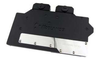
The Koolance VID-NX980 is a full coverage video block for water cooling NVIDIA reference GeForce GTX 980 cards in single and multi video card configurations. It utilizes a high-performance microfin (0.5mm) design made of solid copper with anti-corrosive nickel plating. Fitting threading is standard G 1/4 BSPP. For multiple card configurations, video connectors are also available.
