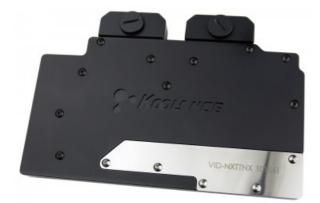
The Koolance VID-NXTTNX is a full coverage video block for water cooling NVIDIA reference GeForce GTX 980 Ti and GTX TITAN X cards in single and multi video card configurations. It utilizes a high-performance microfin (0.5mm) design made of solid copper with anti-corrosive nickel plating. Thermal interface material and mounting hardware are included. Tube fitting threads are G 1/4 BSPP.
