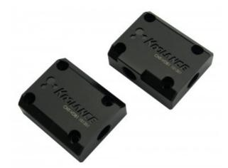
Koolance video bridge connectors link multiple video water blocks together with ease. Flow can be directed in series or parallel. CNT-VDB1 is for combining two (dual L-bracket) video blocks which are in consecutive PCI-Express slots. This product is only compatible with Koolance VID-series water blocks which have detachable fitting bases (launched in 2013 or later).
