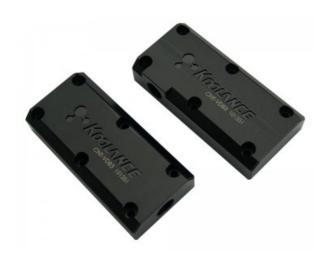
Koolance video bridge connectors link multiple video water blocks together with ease. Flow can be directed in series or parallel. CNT-VDB3 is for combining three (dual L-bracket) video blocks which are in consecutive PCI-Express slots. This product is only compatible with Koolance VID-series water blocks which have detachable fitting bases (launched in 2013 or later).
