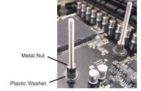
plastic washer around each mounting post. Hand-tighten a metal nut onto each post above the washer to hold the rear bracket in place.
