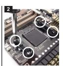
(AMD boards only) AMD sockets require removal of the motherboard's existing retention frame in order to install the Koolance water block.
