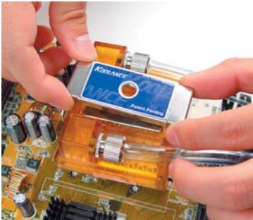
Clips for AMD socket 472 & Intel P-III socket 370
