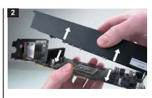
With all screws removed, carefully remove the card heat sink. Original thermal paste may present resistance during removal.
