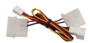
3-pin to 4-pin Molex fan or pump power adapter. Both male and female plugs are provided with 3-pin and 4-pin connections. Can also be used to combine tachometer and power wires of PMP-450/S pumps into a single 3-pin plug. 36cm (14in) in length.
