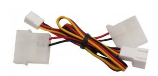
3-pin to 4-pin Molex fan or pump power adapter. Both male and female plugs are provided with 3-pin and 4-pin connections. Can also be used to combine tachometer and power wires of PMP-450/S pumps into a single 3-pin plug. 36cm (14in) in length.
