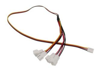
Four 3-Pin female fan connections combine into a single 3-pin male connection. For combining or extending radiator fans. One of the connections features a tachometer wire that is extended to the male connection. Approximately 24" (31cm) long.
