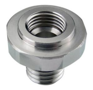
ADT-XFTK is a G 1/4 BSPP female threaded fitting for installation into a panel or reservoir. It is self-sealing with the included EPDM o-ring. A stainless steel washer and nut for the rear side are included.
