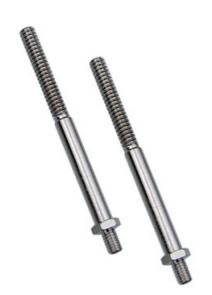
Threaded mounting bolts for the Koolance CPU-360, CPU-370, and CPU-380 to fit socket AMD G34 processors with a fixed back plate (such as with the Supermicro MBD-H8SGL-F-O). These two bolts screw directly into the stock motherboard backplate.
