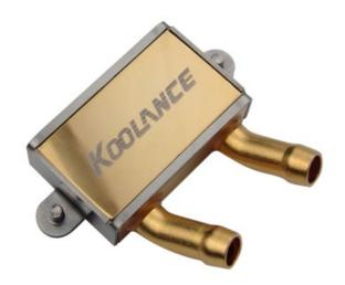
The CHC-35-D06 is for GeForce 7800/7900 GTX voltage regulator circuits. It is a high density copper block with 24k gold plating inside and out. It replaces the rear "VREG" heat sink of 7800GTX and 7900GTX video cards when liquid cooling the main GPU (which removes the default air flow).
