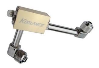
The CHC-37-L06 is for GeForce 7800/7900 GTX voltage regulator circuits. It is a high density copper block with rotational L-fittings and 24k gold plating inside and out. It replaces the rear "VREG" heat sink of 7800GTX and 7900GTX video cards when liquid cooling the main GPU (which removes the default air flow).
