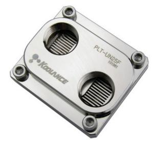
PLT-UN25F is a high-efficiency, general-purpose cold plate for thermal applications such as TEC, LED, image sensor, and semiconductor cooling. The active cooling area is 25mm x 25mm (0.98in x 0.98in), and it utilizes a 0.5mm microfin internal structure.
