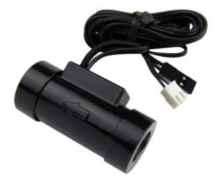
Koolance's inline flow meters provide electronic indication of real-time coolant flow rate. This model uses a reed switch to detect impeller rotation, and integrates a thermistor coolant temperature sensor (10K Ohms @ 25°C). G 1/4 BSPP fitting threads, and primary materials are a stainless steel body with brass threads. Approximate read range is 2.0-20 LPM (32-317 GPH). Wire length is about 28" (70cm). It is recommended to keep current through the flow meter at 10mA or less to prevent damage.
