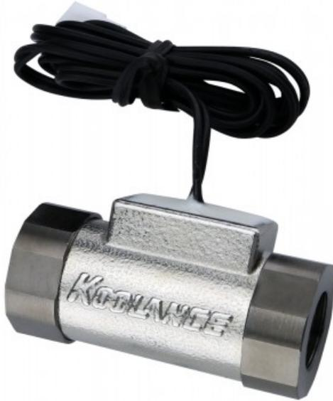
Koolance's inline flow switch provides a simple electronic confirmation of coolant flow. The switch will close if the flow rate stays above 2.0LPM / 0.53GPM (+/-10%), and opens when below. Fitting threads are G 1/4 BSPP, and the primary materials are stainless steel and nickel-plated brass. Wire length is about 28" (70cm). It is recommended to keep current through the flow switch at 10mA or less to prevent damage.
