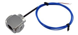
Coolant K-type thermocouple temperature sensor with fitting body. This product is designed to be placed inline on any hose. Simply choose G 1/4 BSPP threaded fittings for the desired hose diameter. Wire length = 30" (76cm). Accuracy =  $\pm$ /-1.5 °C, temperature range = -40 to 120 °C (-40 to 248 °F).
