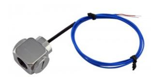
Coolant K-type thermocouple temperature sensor with fitting body. This product is designed to be placed inline on any hose. Simply choose G 1/4 BSPP threaded fittings for the desired hose diameter. Wire length = 30" (76cm). Accuracy =  $\pm -1.5$ °C, temperature range =  $\pm 0$ 0 to  $\pm 0.24$ °C.
