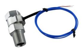
Coolant thermocouple temperature sensor within a swiveling brass body. Male and female NPT 1/4" threads are provided on either end. Wire length = 30" (76cm). Accuracy = +/- 1.5 °C, temperature range = -40 to 120 °C (-40 to 248 °F).
