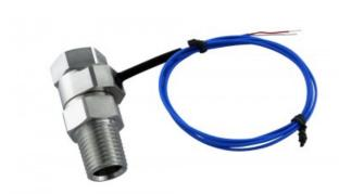
Coolant thermocouple temperature sensor within a swiveling brass body. Male and female NPT 1/4" threads are provided on either end. Wire length = 30" (76cm). Accuracy = +/- 1.5 °C, temperature range = -40 to 120 °C (-40 to 248 °F).
