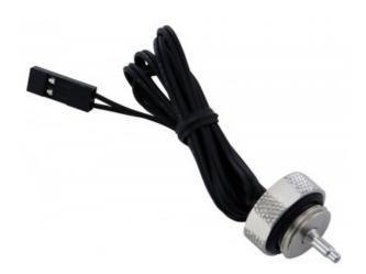
Coolant thermistor temperature sensor compatible with Koolance multi-sensor systems. Sensor fitting is G 1/4 BSPP (parallel) threaded. Wire length = 30" (76cm). NOTE: This sensor will only work with Koolance products which use 10K Ohm @25°C sensors (first introduced in 2011).
