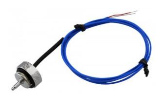
Coolant K-type thermocouple sensor, compatible with Koolance EXC and ALX series systems. Sensor fitting is G 1/4 BSPP (parallel) threaded. Wire length = 38" (965mm). Accuracy =  $\pm$ 1.5°C, temperature range = -40 to 120°C (-40 to 248°F).
