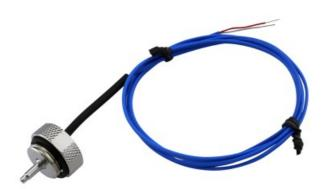
Coolant K-type thermocouple sensor, compatible with Koolance EXC and ALX series systems. Sensor fitting is G 1/4 BSPP (parallel) threaded. Wire length = 38" (965mm). Accuracy =  $\pm -1.5$  °C, temperature range =  $\pm 40$  to  $\pm 120$  °C ( $\pm 40$ to 248°F).
