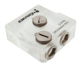
COV-PMP400AC is an acrylic fitting base for the Koolance PMP-400 pump (sold separately). Along with enabling the use of any G 1/4 BSPP (parallel) thread fitting style and diameter, it allows flow to be specifically directed for increased pump performance, or broader chassis integration.
