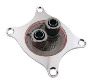
The high flow, all-purpose CPU-345 improves upon Koolance's patented design with increased surface area and better coolant flow positioning. Materials include a high-density solid copper cold plate, anti-corrosive nickel plating, and a transparent acrylic (model CPU-345AC) or opaque acetal (model CPU-345AT) top.
