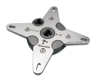
Following the extremely successful CPU-350 comes Koolance's latest high-performance CPU water block. The CPU-360 uses an advanced microfin cold plate (0.25mm fins, 0.30mm channels), o-ring sealed impingement plate, and an optimized flow path to yield best performance with relatively low coolant restriction.
