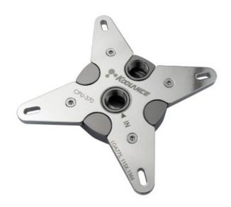
The CPU-370 contains an advanced microfin cold plate (0.25mm fins, 0.30mm channels), o-ring sealed impingement plate, and an optimized flow path minimize coolant restriction.
